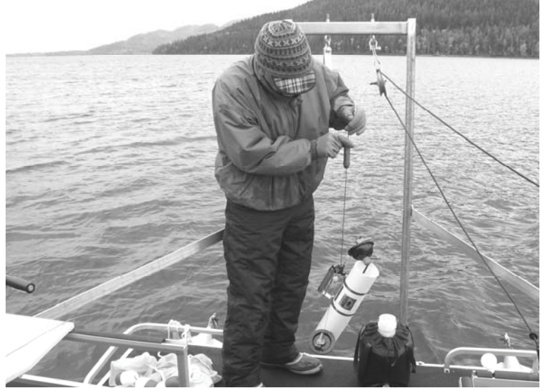
Scientist Chris Ruffatto reads a VanDorn water sampler during a crisp autumn day on the lake. A messenger (held in Chris' right hand) is sent down the steel cable to trigger a button on the VanDorn sampler, closing both ends. The sampler allows water quality samples to be collected at specific depths in the lake.
