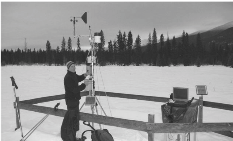
Mike Koopal makes adjustments to the WLI weather station after bitterly cold weather in December took its toll on the batteries.
